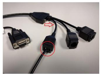
2. Attach the RJ-11 connector to the COM1 RS232 port. If you have an interface cable with colored tips it is the BLUE connector, otherwise attach it to the RS232 port that is closest to the power adapter input.
