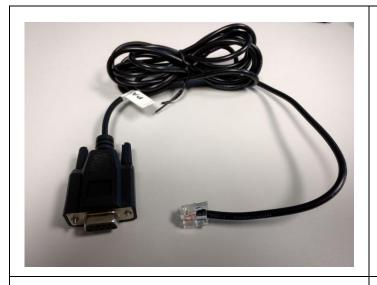
1. Locate the cable with a 9-hole serial connector and an RJ-11 connector that was included with the PAX device.
