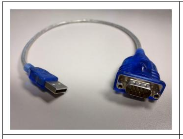
1. Locate the Cables to Go serial to USB adapter; Model: 26886; UPC-A: 757120268864.
