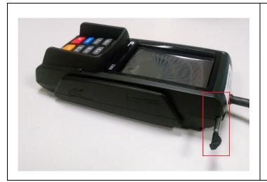
The stylus can be found inserted horizontally on the top right of the PAX.
