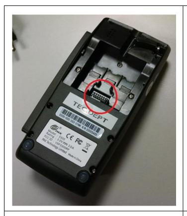
1. Remove the back cover from the PINpad and locate the 14-pin connector.
