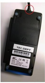
8. Replace the back cover making sure to properly align the cable grommet into the channel.
