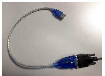
2. Connect the 9-pin adapter to the 9-hole adapter on the Serial cable.
