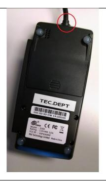
8. Replace the back cover making sure to properly align the cable grommet into the channel.
