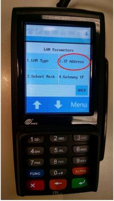
8. Tap on **IP Address** or press **2** on the keypad.
