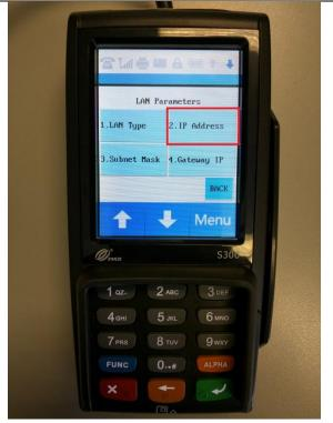
8. Tap on **IP Address** or press **2** on the keypad.
