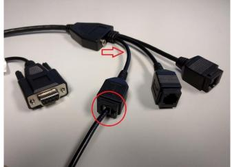
2. Attach the RJ-11 connector to the COM1 RS232 port. If you have an interface cable with colored tips it is the BLUE connector, otherwise attach it to the RS232 port that is closest to the power adapter input.
