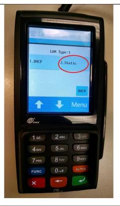
11. Tap on **Static** or press **2** on the keypad.
