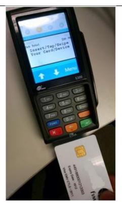
3. Insert the EMV Chip card into the slot on the bottom of the S300.
