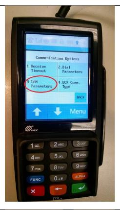
7. Tap on **LAN Parameters** or press **3** on the keypad.
