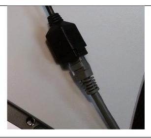
6. Connect an Ethernet cable (with internet) to the port on the data/power cable that says "LAN". (The other 2 connections are not used.)
