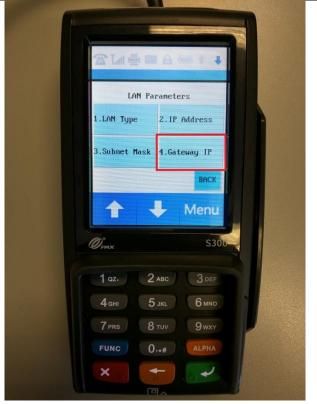
11. Tap on **Gateway IP** or press **4** on the keypad.
