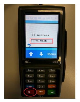
8. Make a note of the **IP Address** then hit the red X key twice to return to the **LAN Parameters** screen.
