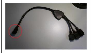
2. Locate the included data/power cable and attach the single end to the 14-pin connector on the PINpad device.
