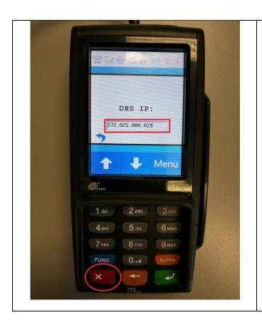
14. Make a note of the **DNS IP**then hit the red X key 5 times
