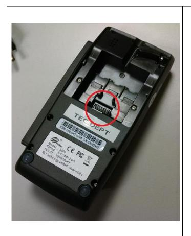
Remove the back cover from the PINpad and locate the 14pin connector.
