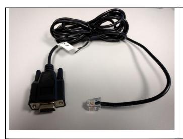
Locate the cable with a 9-hole serial connector and an RJ-11 connector that was included with the PAX device.
