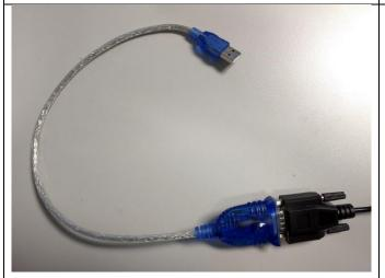
2. Connect the 9-pin adapter to the 9-hole adapter on the Serial cable.
