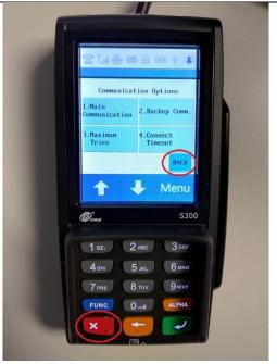
10. Tap on the **BACK** button, or press the red key on the keypad until you are back at the main screen.
