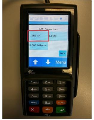
13. Tap on **DNS IP** or press **1** on the keypad.
