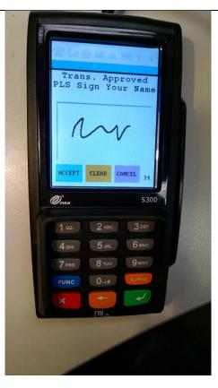
5. Sign on the screen using a finger or the S300 stylus then hit the **ACCEPT** button.
