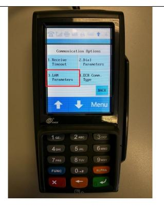
7. Tap on **LAN Parameters** or press **3** on the keypad.
