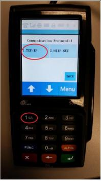
10. Tap on **TCP/IP** or press **1** on the keypad.
